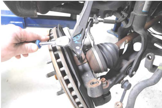
10. Using a 10mm socket, remove the ABS sensor from the knuckle. Retain the hardware for re-use.
