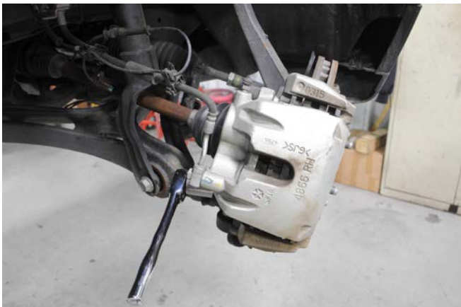
11. Using a 21mm socket, remove the brake caliper and hang the caliper out of the way. Retain hardware for re-use. Do not hang caliper by the brake line
