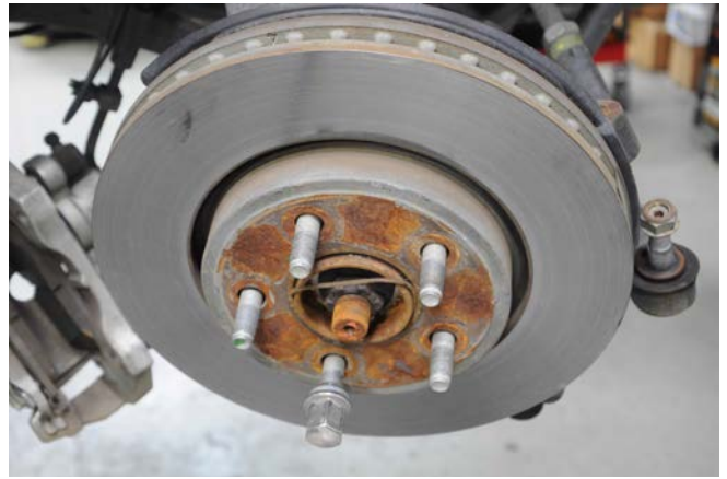
13. Using a 32mm socket, remove the axle nut. Retain for re-use.
