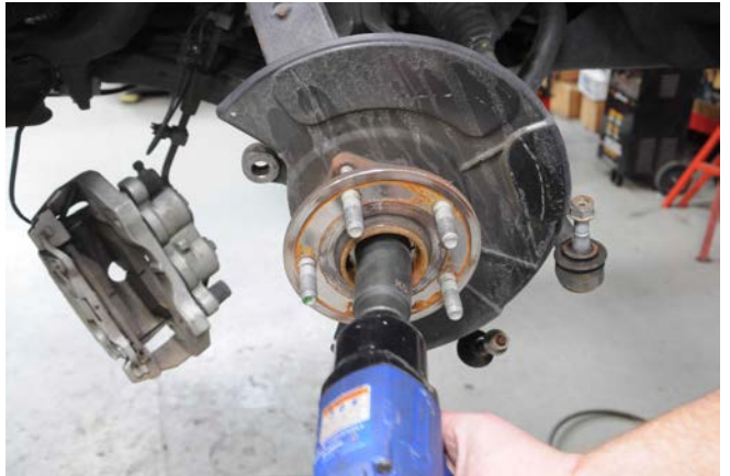
13. Using a 32mm socket, remove the axle nut. Retain for re-use.
